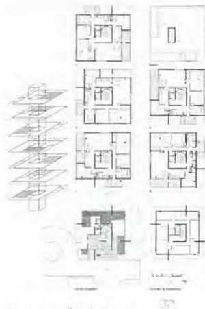
FIGURE 2. Atelier de Montrouge, EDF staff housing towers, Ivry-sur-Seine, 1963-67. Layout of the small tower and construction system. © SIAF/CAPA/Archives d'architecture du XX e siècle, ATM.
